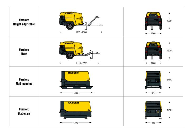
unbraked chassis and height adjustable tow bar
